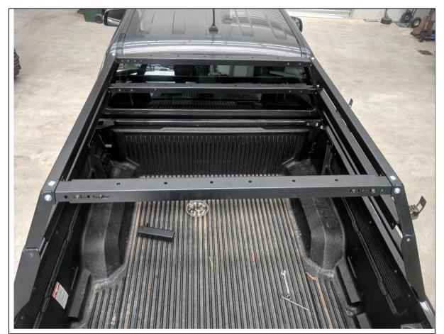
12. With Assistance lift the height extension onto the existing base rack.
