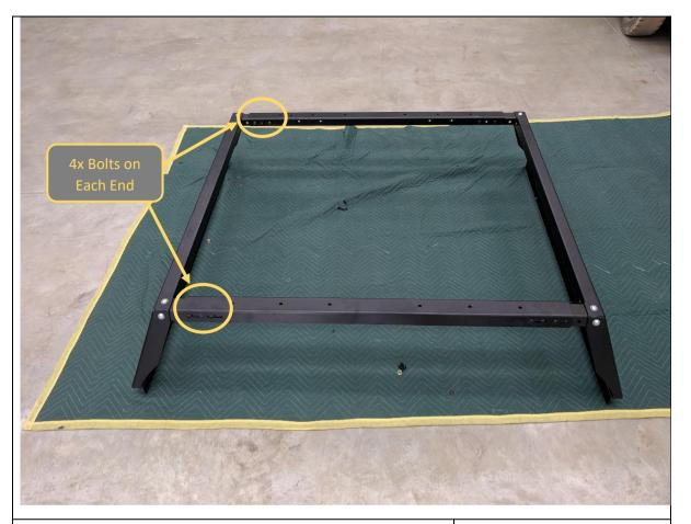
8. Lift up cross bars onto opposite side knuckles. Secure with 8x M8x20 Button Head bolts, Flat washers and flange nuts.
