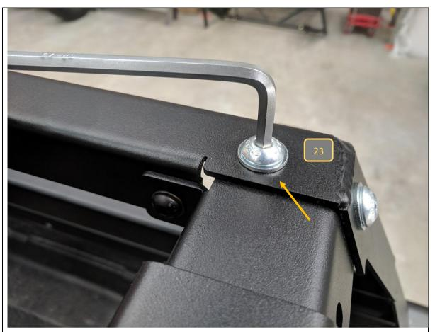
23. Tighten all bolts connecting the side lowers to the cross bar knuckles, using 6mm Hex key and 15mm spanner.
