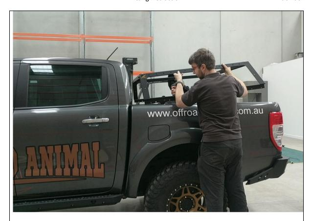
9. With assistance, Lift the assembled tub rack onto the bed of the ute.
